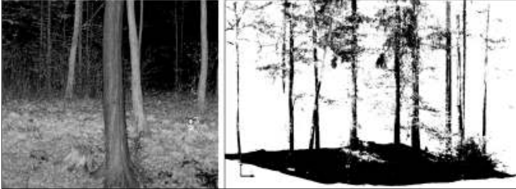
Figure 2. Fragment of forest stand LIDAR image based on the cloud of points and LIDAR image with photography superimposed
