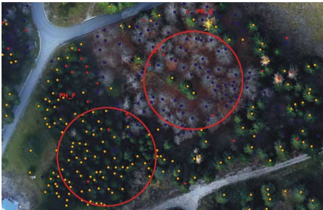
Figure 3. Examples of single tree extraction and species classification results in two leaf-off plots (PH_F and PH_E, from the left to the right). Spruces, larches and birches are colored in yellow, red and blue, respectively
