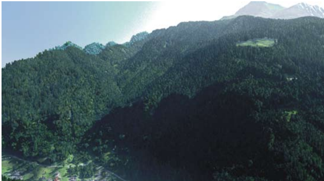
Figure 4. Photorealistic rendering in a forestry study area (Pramosio, Udine) obtained by the integration of LIDAR DTM (Digital Terrain Model) and LIDAR-extracted forestry parameters and digital orthophotos (image elaborated by means of VNS software).
